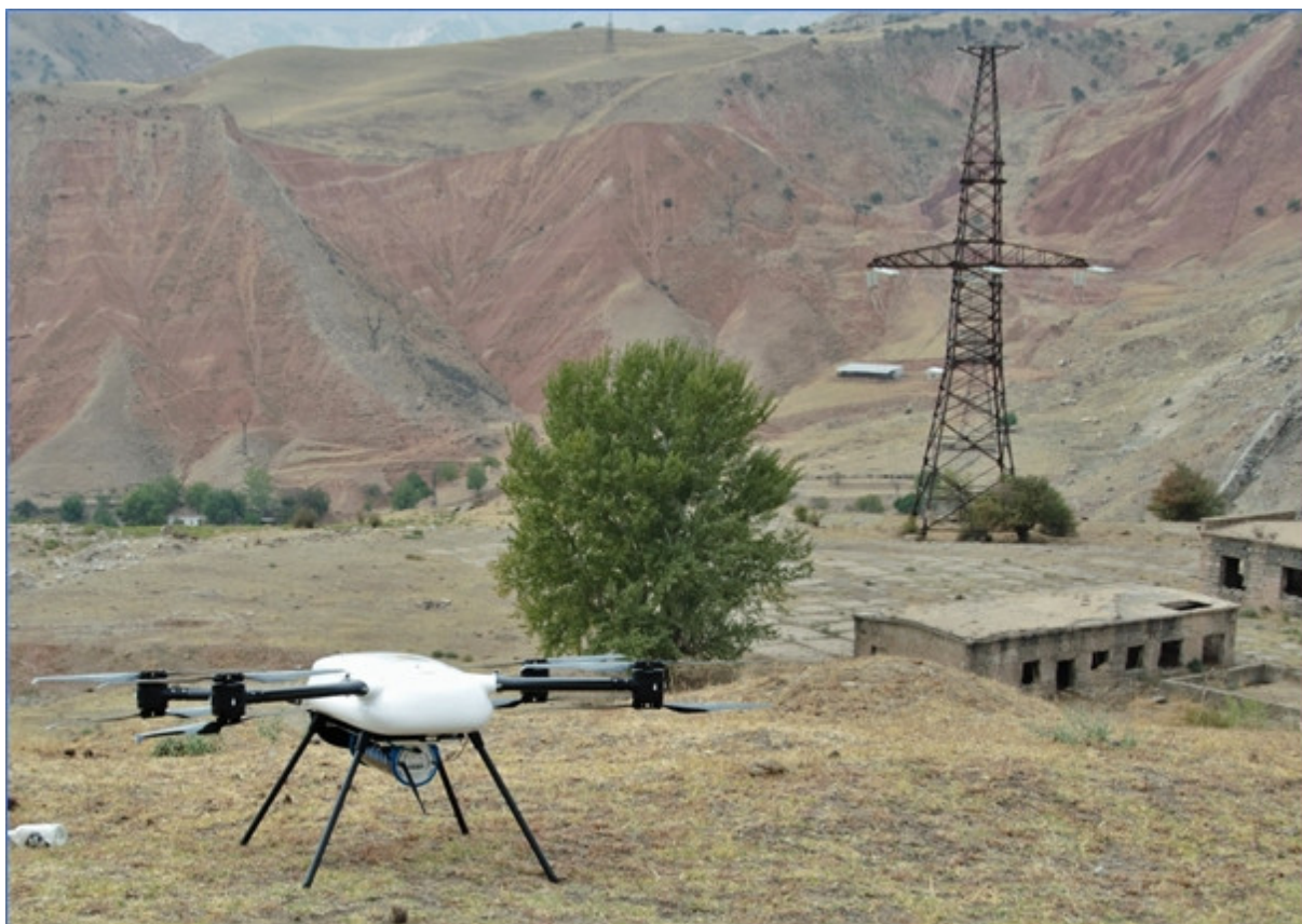
Figure 1. View of the UAV: note the gamma spectrometer mounted from below to the drone.
